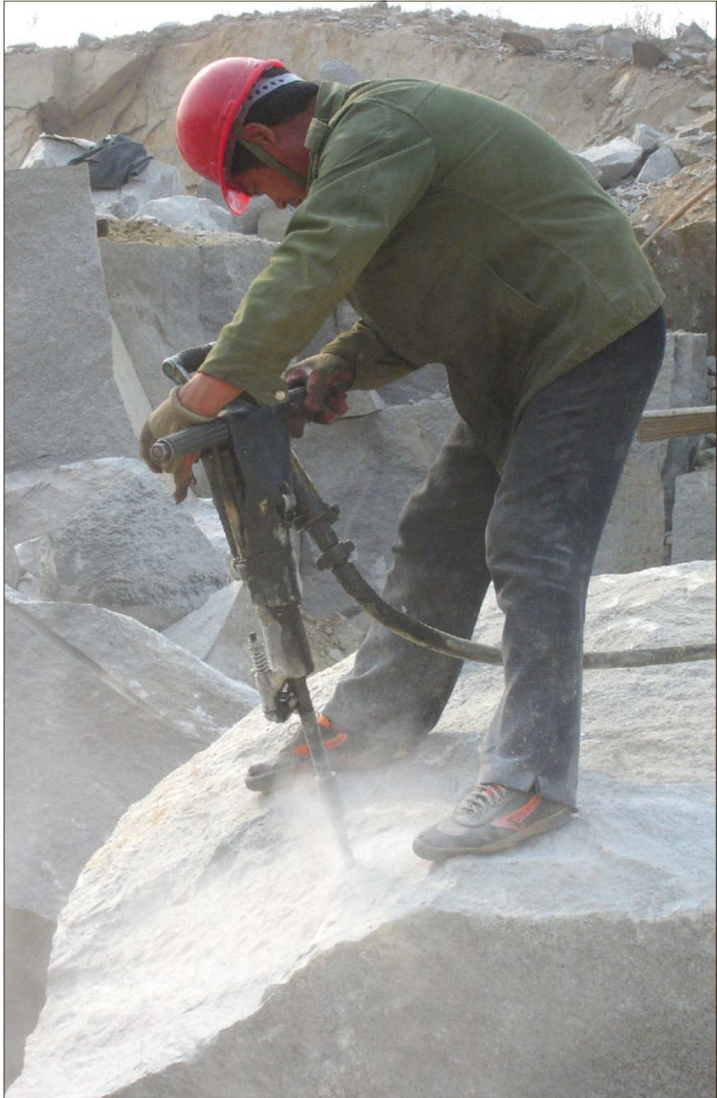
At the time of our visit one worker is drilling a large granite block causing a dust cloud to rise up into the air. He is using no protective equipment, neither a face mask nor ear plugs.
