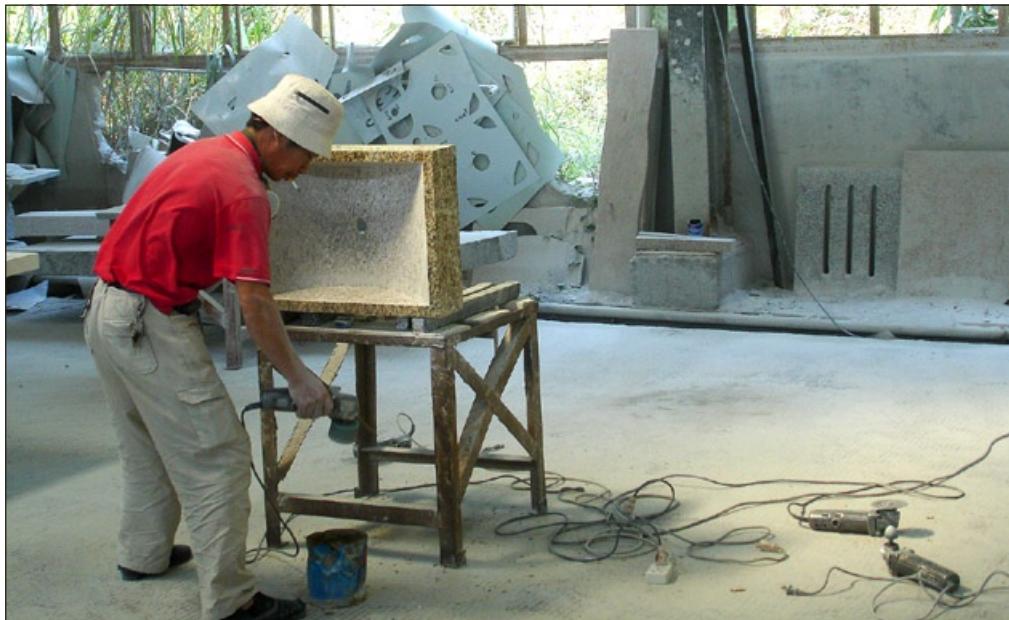
A worker at Supplier C is making bathroom sinks, creating a smooth basin shape with a special handheld machine. This job generates a lot of dust. He is wearing a special face mask with inhalation and exhaust valves and filters, but the type of filters could not be checked. However, the worker removed the mask every now and then to smoke a cigarette.
