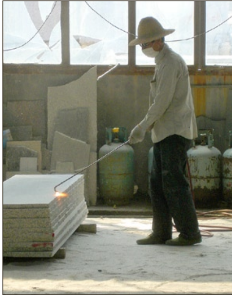
A worker wearing a cloth face mask is flaming stone inside the factory hall at Supplier C. During measurements in flaming operation outdoors in Swedish stone industry the level of quartz dust was found to be six times higher than the Swedish legal level requires. For this operation the worker should use both a dust respirator and protective mask with P3 filter.
